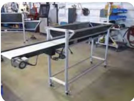
Conveyor with Hopper
