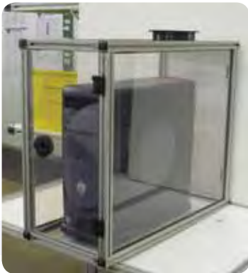
Computer Enclosure with HEPA Filter and Fan
