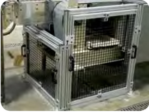
Conveyor Lift Off Perimeter Guard
