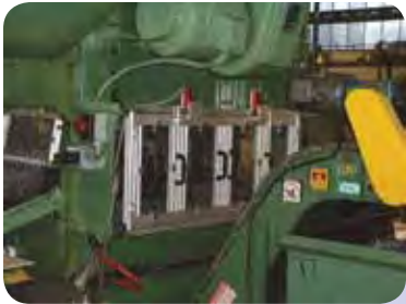
Bi-fold Guard on Back Side of Press
