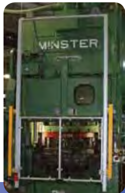
Safety Press Guard with Light Curtains
