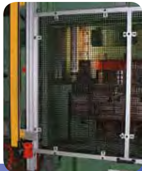
Press Guard with Light Curtain and Safety Interlock
