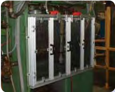
Bi-fold Guard with Safety Interlocks
