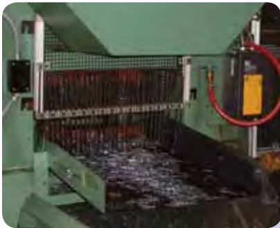
Chute Guard with Adjustable Fingers
