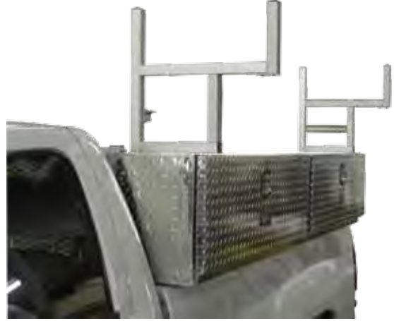
Ladder rack brackets for installation truck
